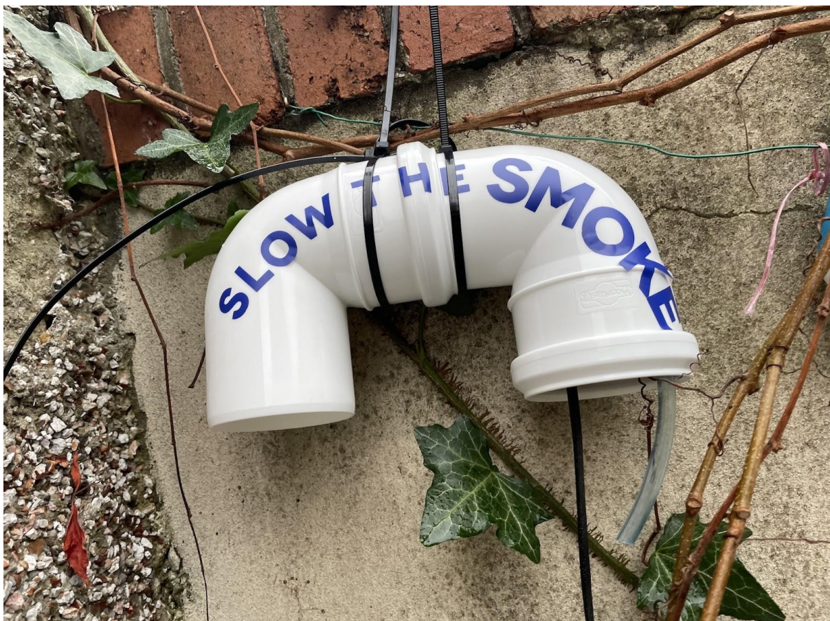
Figure 21. One of the Slow the Smoke air quality sensors used by citizen scientists
